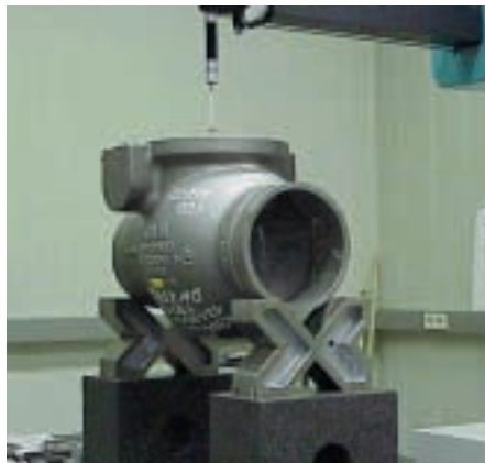
SCV body during ISO Certification on the 3D measuring machine
