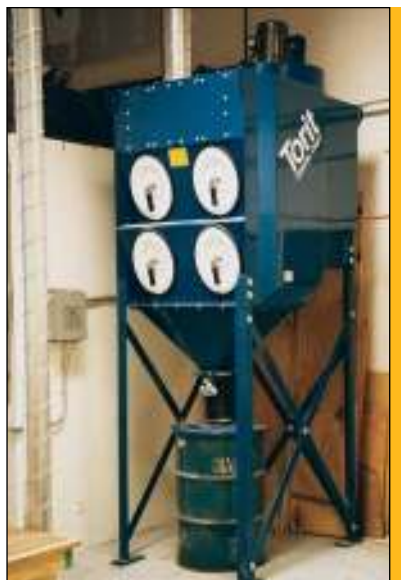
DFO 2-4 on fiberglass routing & cutting
